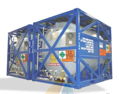
The ISO-PACK 20<mark>00 6bar is a vacuum insulated liquid gas transportable / storage tank, designed to transport liquid Nitrogen by road, rail and sea. The tank dimensions meet</mark>
